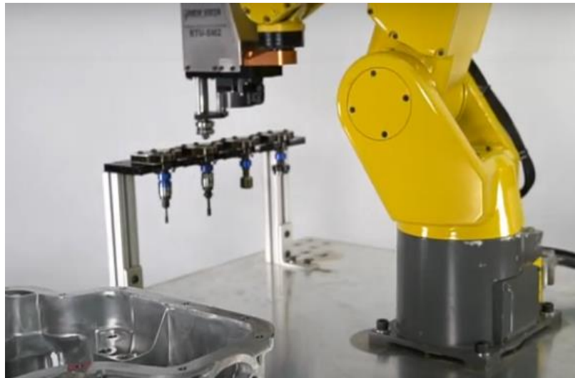
This standard-issue, servo-driven RTU is equipped with the Type J Auto-change Chuck, for use in conjunction with the New Vista Type J Tool Docking System.
